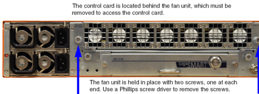
Figure 1 Replacing a Control Card
