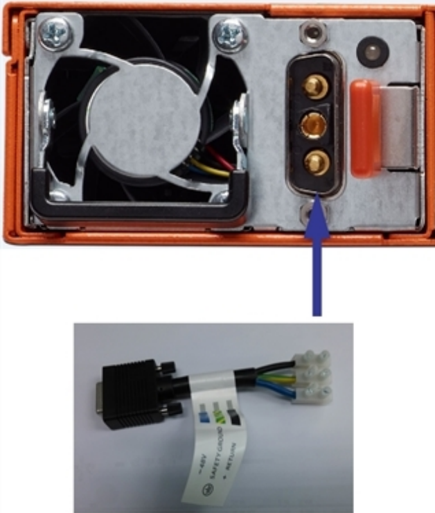
Figure 4 DC Power Module
