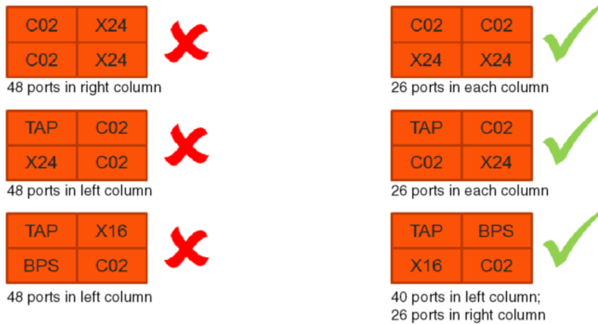
Figure 7 Module Placement of PRT-HC0-CO2, 100G Mode
